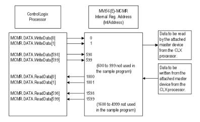
The sample configuration values configure the module database for **WRITEDATA[0 TO 599]** to be stored in the module memory at register 0 to 599, and **READDATA[0 TO 599]** to be stored in the module memory at registers 1000 to 1599 as shown above.
