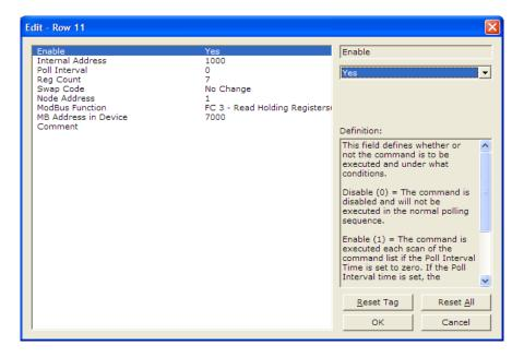
Notice that the count is now set to a value of 7. Because the Slave device utilizes only 7 Modbus addresses, a count of 7 will cause the Slave to respond with 14 registers (28 bytes) of information.
