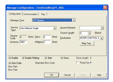
A 5-word response will be passed back through the MSG instruction to the controller tag array, **MCMR.CONTROL.EVENTCMDRESPP1**. or **MCMR.CONTROL.EVENTCMDRESPP2**, depending on whether the Event Command was sent for Port 1 (**9901**) or Port 2 (**9911**). The following table lists the 5-word response data received:
