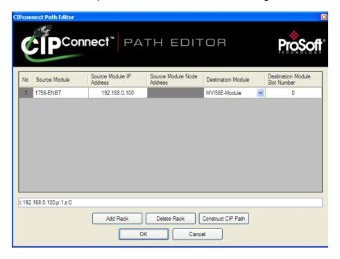
The CIPconnect Path Editor allows you to define the path between the PC and the MVI56E-MCMR module. The first connection from the PC is always a 1756-ENBT (Ethernet/IP) module.
