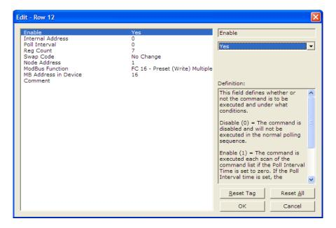
Based on the Internal Address and the configuration within the **BACKPLANE CONFIGURATION** section for Write Register Start and Write Register Count, the data from the tag **MCMR.DATA.WRITEDATA[0]** To [6] will be written to Modbus addresses 47001 to 47007 of Modbus Slave Device Address 1.
