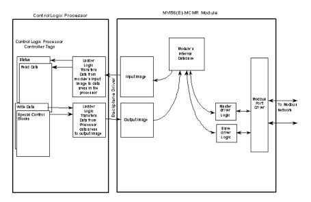
As shown in the diagram, all data transferred between the module and the processor over the backplane is through the Input and Output Images. Ladder logic must be written in the ControlLogix processor to interface the Input and Output Image data defined in the controller tags. The user is responsible for handling and interpreting all data received on the application ports and transferred to the Input Image.
