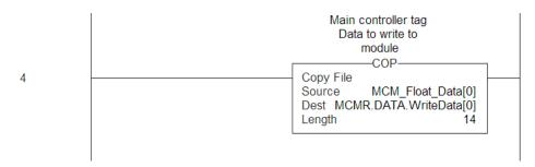
2 The length of this COP statement must now be 14. This will COP as many of the MCM\_FLOAT\_DATA values required to occupy the MCMR.DATA.WRITEDATA array for a length of 14. This will take 7 registers, MCM\_FLOAT\_DATA[0] TO [6], and place that data into MCMR.DATA.WRITEDATA[0] TO [13].
