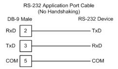
**Note:** For most null modem connections where hardware handshaking is not required, the *Use CTS Line* parameter should be set to **N** and no jumper will be required between Pins 7 (RTS) and 8 (CTS) on the connector. If the port is configured with the *Use CTS Line* set to **Y**, then a jumper is required between the RTS and the CTS lines on the port connection.
