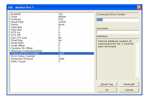
With the **COMMAND ERROR POINTER** set to address 1500, this will place your Command Error Data at addresses starting at 1500 of the module memory, and because of the before mentioned configuration of the **BACKPLANE CONFIGURATION READ REGISTER START** and **READ REGISTER COUNT** parameters, the command error data will be placed into the tags beginning at **MCMR.DATA.READDATA[500]**.
