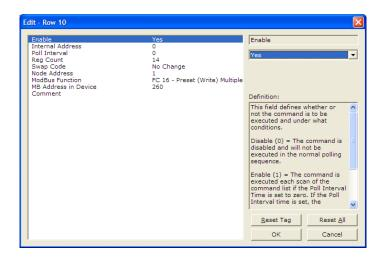
The above command will take the data from **MCMR.DATA.WRITEDATA[0] To [13]** and write this information to Modbus Slave Device Address 1 at data addresses 40261 to 40274.
