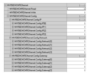
The bit will be automatically reset and the current Ethernet settings will be copied to **MVI56MCMRETHERNET** controller tag as follows.
