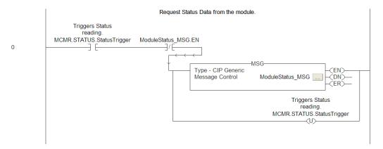
The following illustration shows the format of the MSG block.
